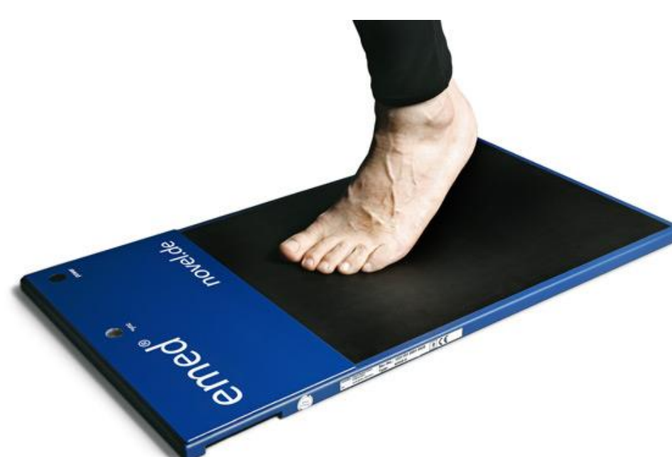
Figure 2 – The pressure matrix (Novel – DE).
